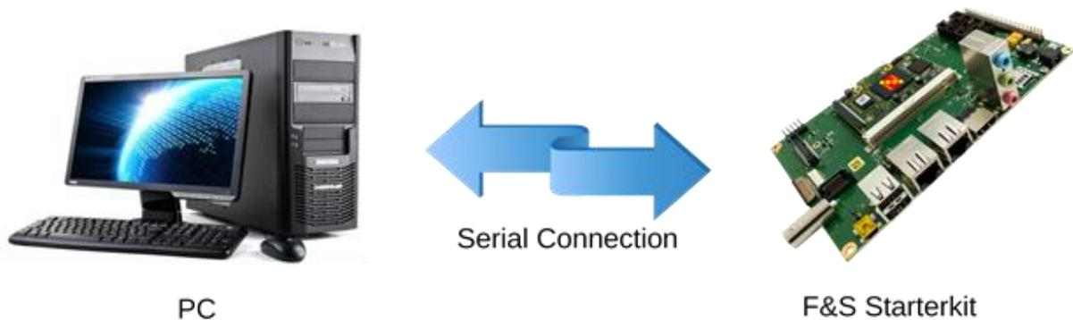
Figure 11: Serial connection from board to PC
