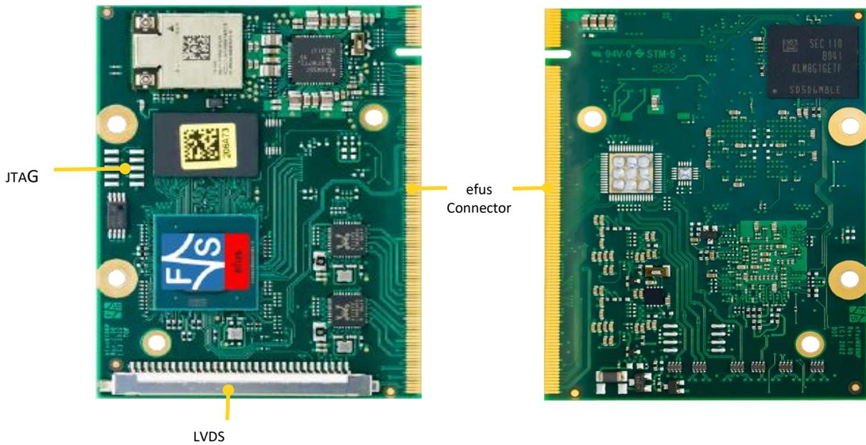
Figure 8: efusMX8MP module top/bottom
