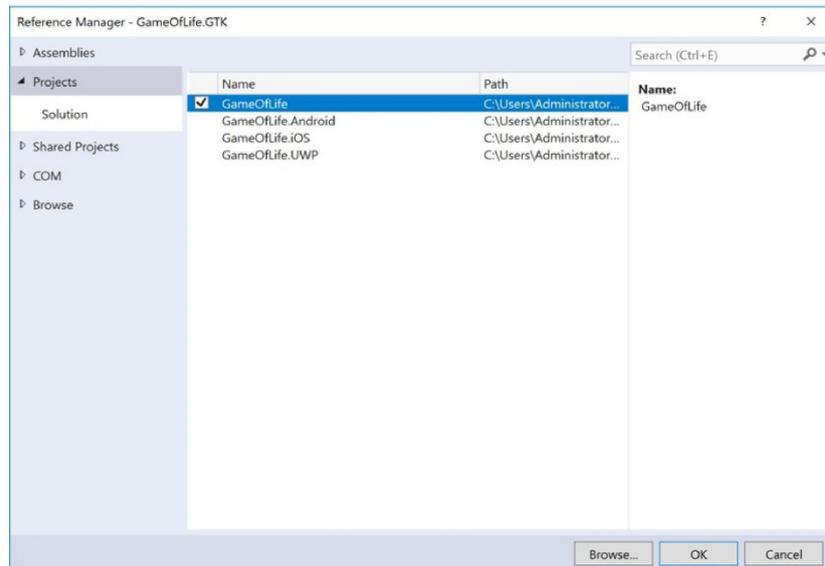
8. In the **Reference Manager** dialog, press the **Browse** button and browse to the **C:\Program Files (x86)\GtkSharp\2.12\lib** folder and select the **atk-sharp.dll**, **gdk-sharp.dll**, **glade-sharp.dll**, **glib-sharp.dll**, **gtk-dotnet.dll**, **gtk-sharp.dll** files.
