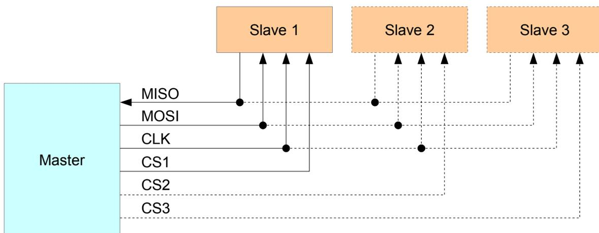
Figure 2: SPI Bus with Master and Three Slaves
