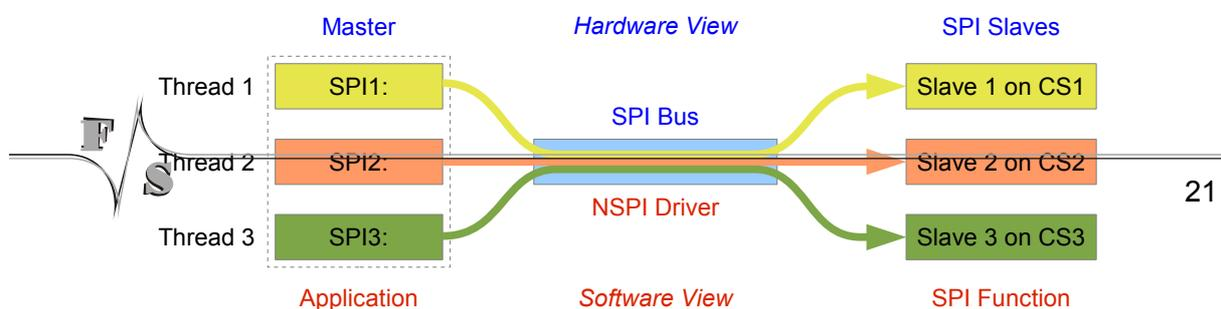
Figure 15: Virtual Connection Between Devices and Slaves
