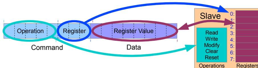
Figure 6: Register Based SPI Device
