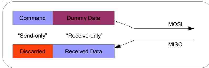
Figure 8: Change of Transfer Direction within an SPI Cycle
