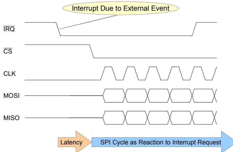
Figure 13: SPI Cycle after IRQ
