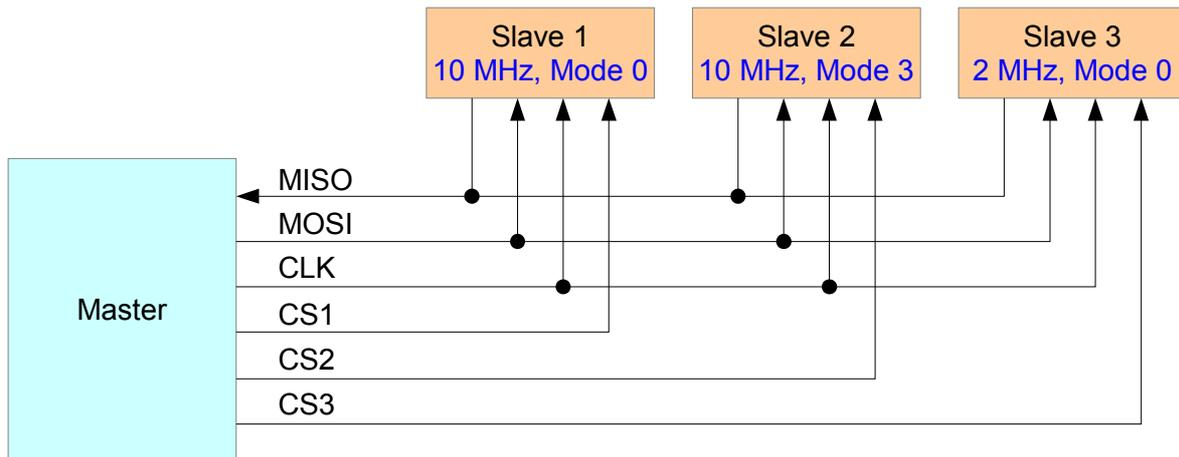
Figure 14: One SPI Bus with Arbitrary Devices
