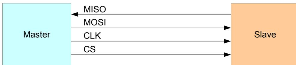
Figure 1: SPI Bus with Master and Slave
