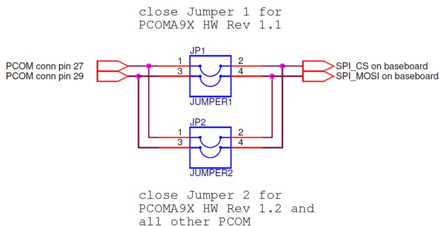
Both pins are configurable as GPIO. In this case this interchange can be handled in SW.
