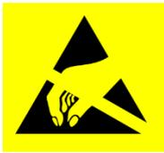
All F&S hardware products are ESD (electrostatic sensitive devices). All products are handled and packaged according to ESD guidelines. Please do not handle or store ESD-sensitive material in ESD-unsafe environments. Negligent handling will harm the product and warranty claims become void.
