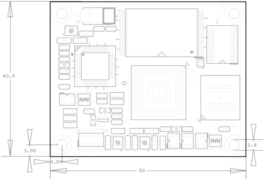
Figure 2: Top view (Mounting holes are isolated from signal ground)
