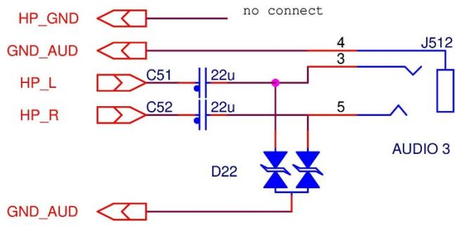
Figure 16 Cap-coupled version of headphone out with GND instead HP\_GND
