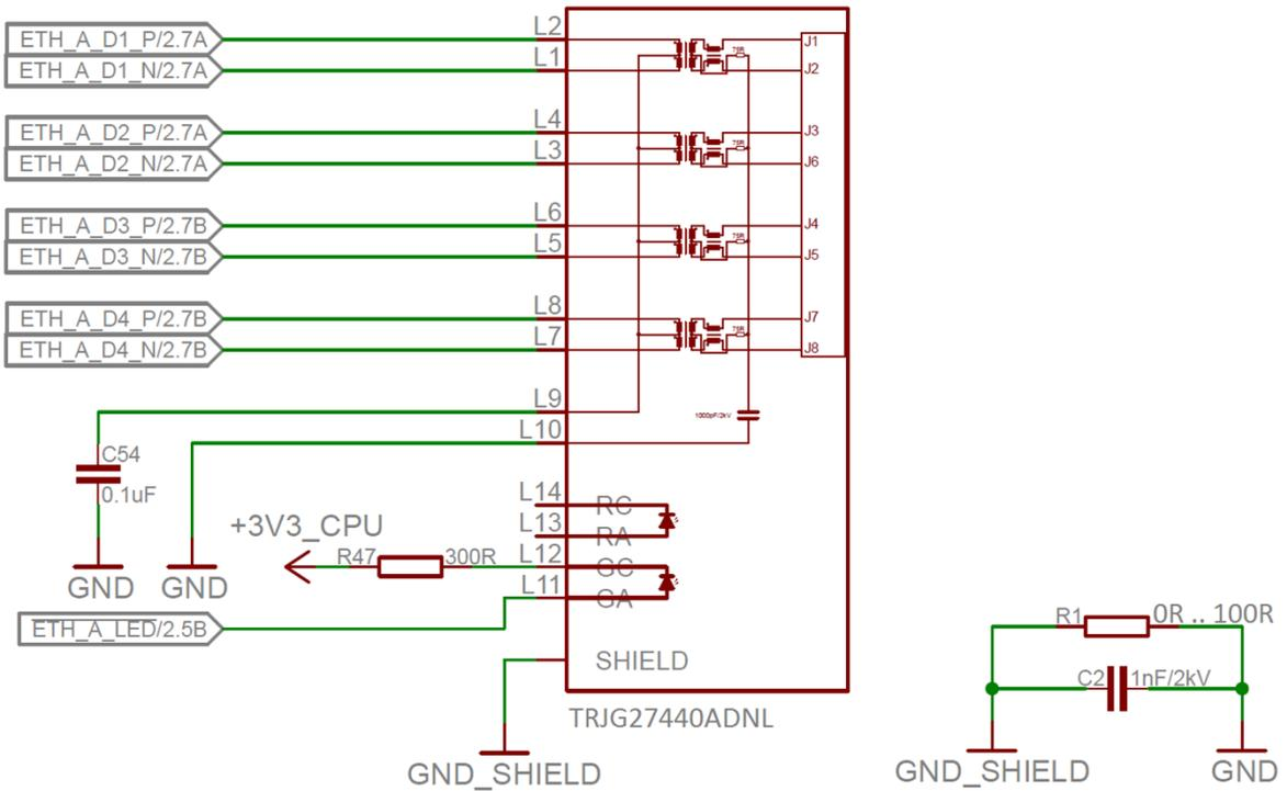
Figure 13: LAN output example
