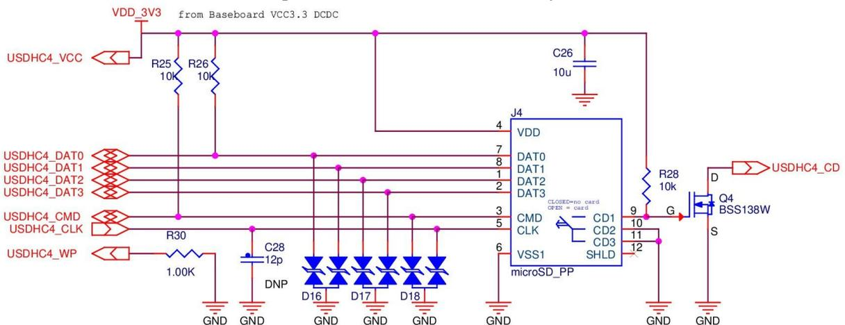
Figure 11: SD basic feature w/o high speed support
