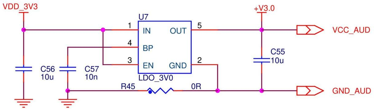
Figure 14: Baseboard LDO power supply for codec analog voltage
