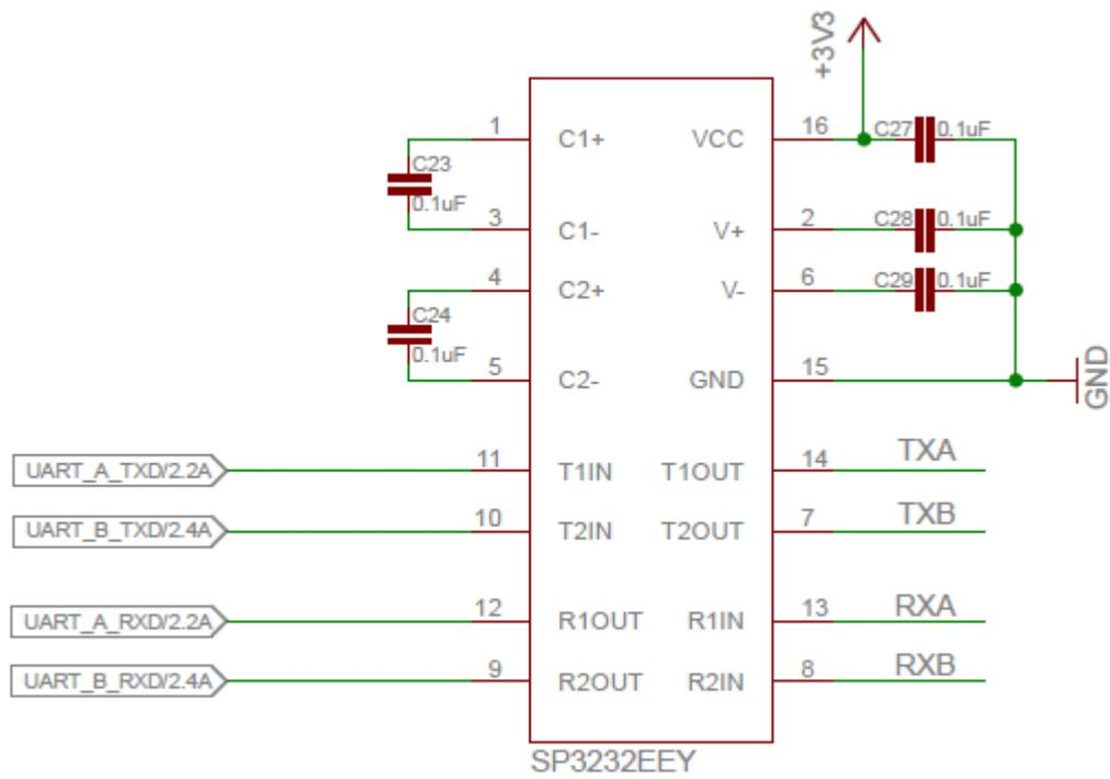
Figure 12: UART transceiver example
