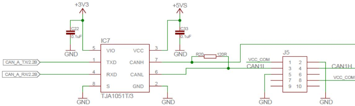
Figure 9: CAN transceiver example
