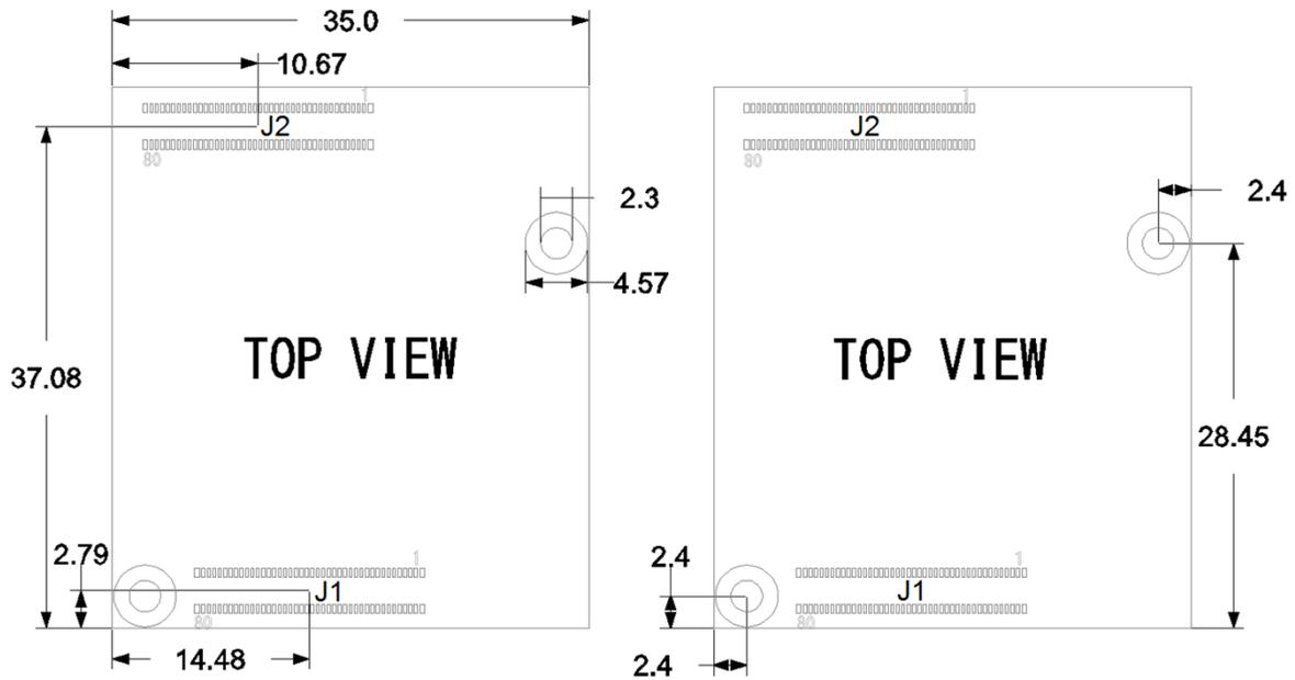
Figure 2: Mechanical Dimension
