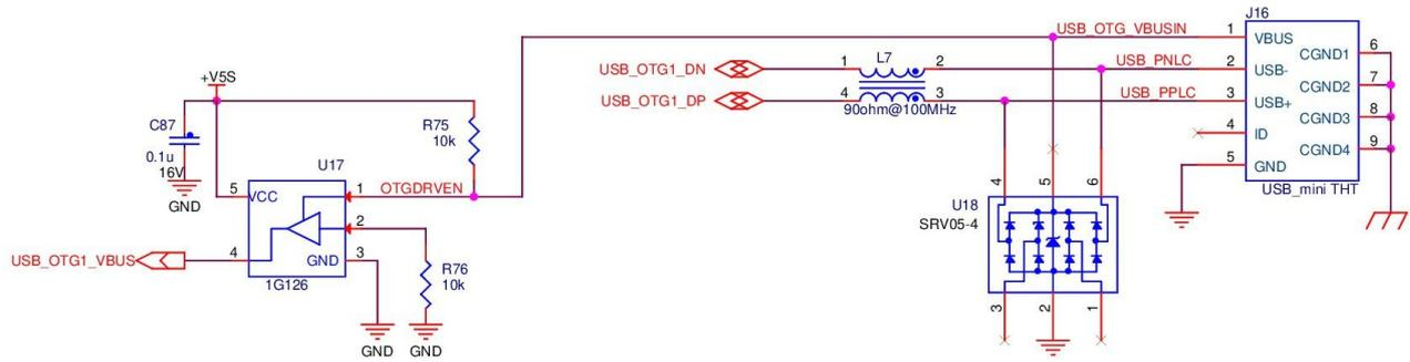
Figure 7: Basic USB Device Example
