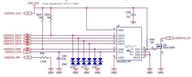
Figure 11: SD basic feature w/o high speed support
