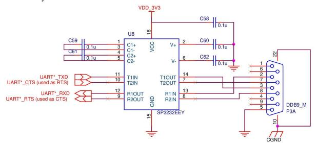
Figure 12: UART transceiver example
