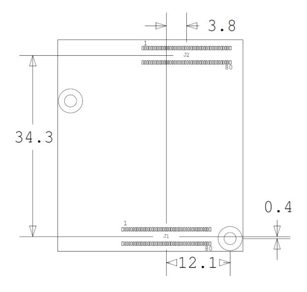
Figure 3: Mechanical Dimensions Bottom
