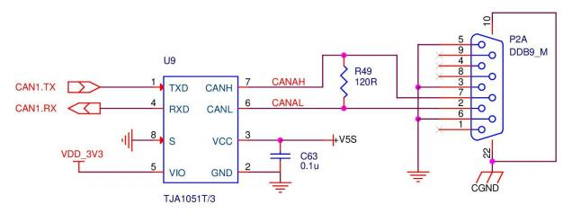
Figure 8: CAN transceiver example
