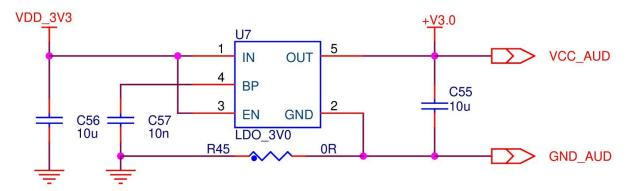
Figure 5: Baseboard LDO power supply for codec analog voltage
