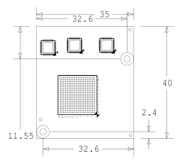
Figure 2: Mechanical Dimensions Top
