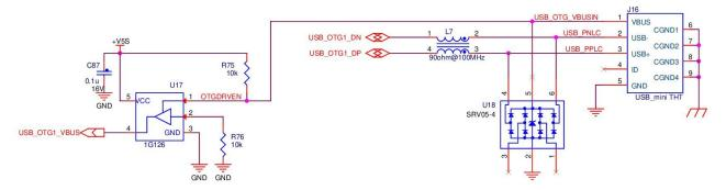
Figure 16: Basic USB Device Example
