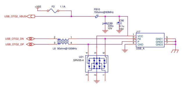
Figure 14: USB Host Basic Feature Example
