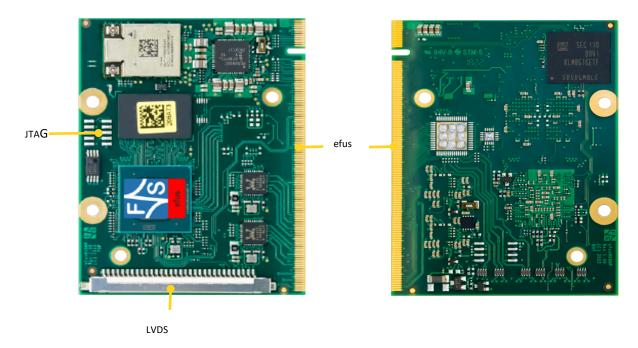
Figure 7: efusMX93 module top/bottom
