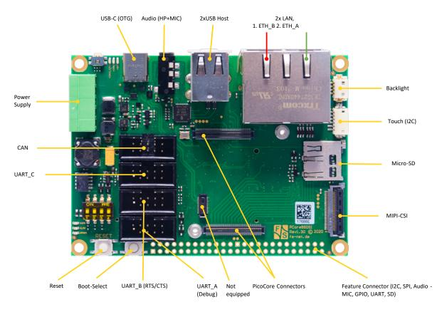
Figure 1: PicoCoreBBDSI Starterkit Top Side (PicCoreBBDSI – Rev. 1.30)
