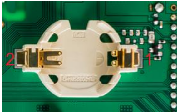
Figure 62: VBAT CR2032 socket
