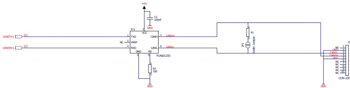
Figure 2: CAN transceiver
