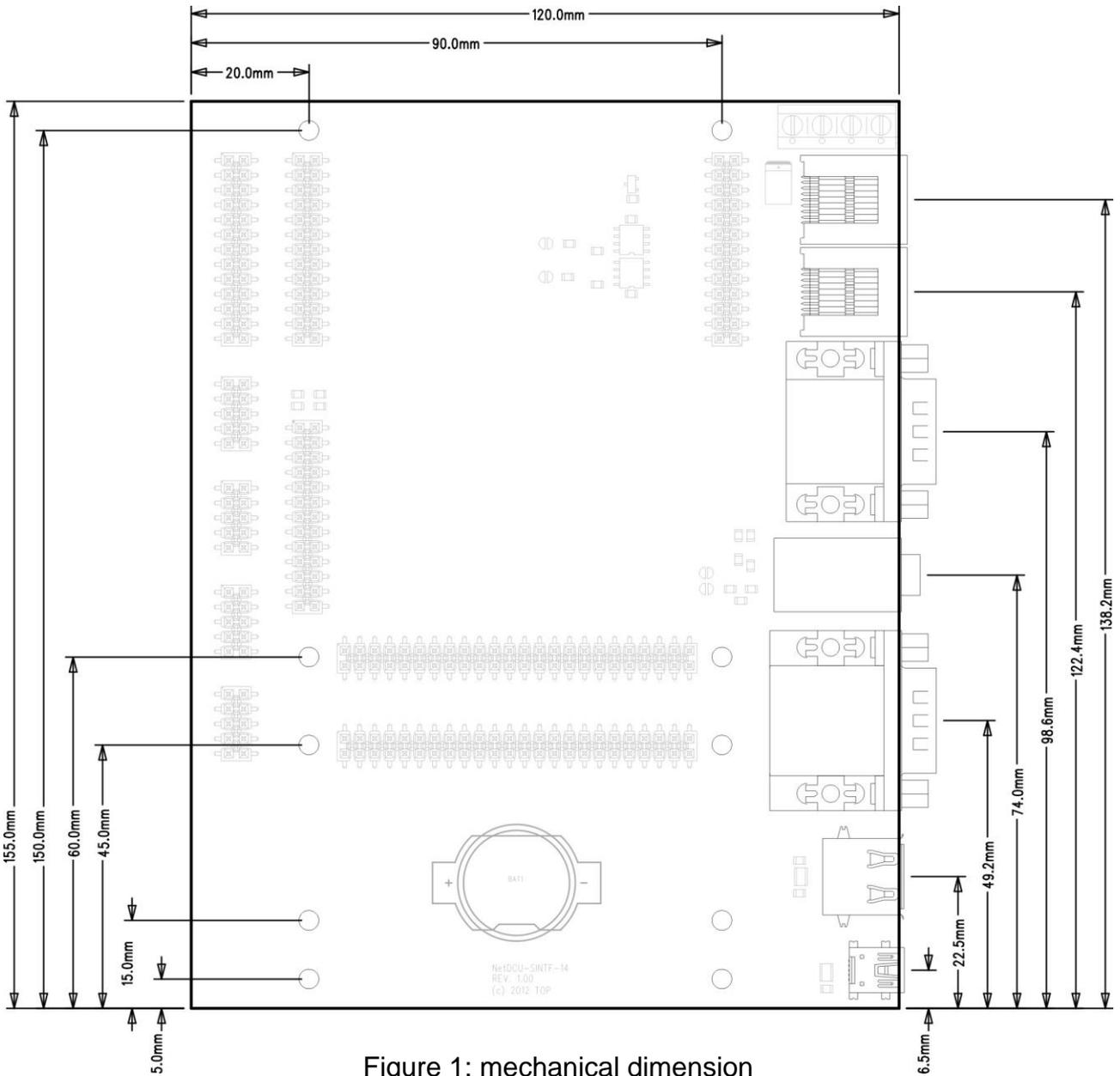
Figure 1: mechanical dimension
