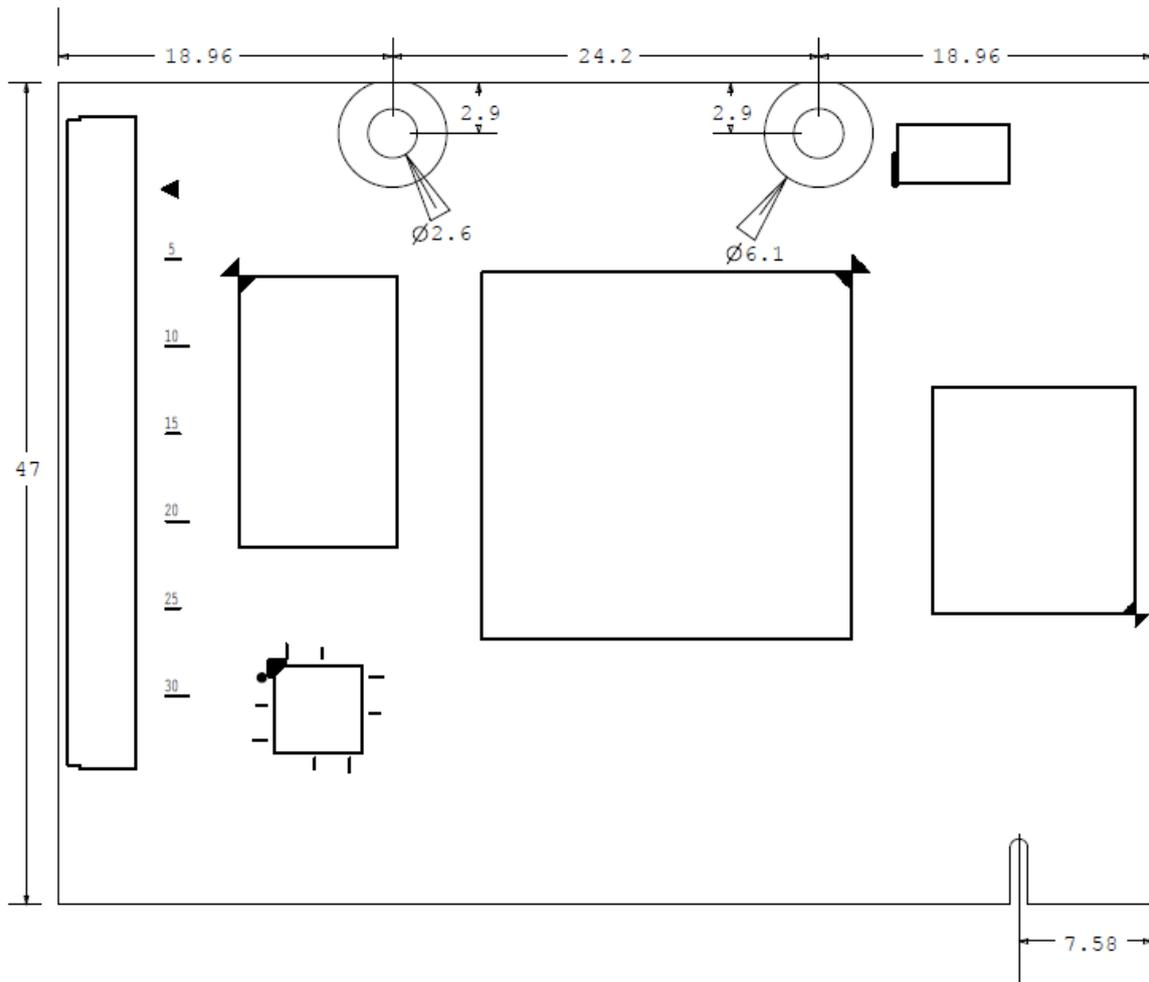
Figure 2: Mechanical dimensions
