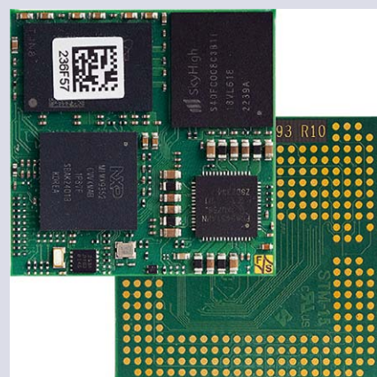
A CoM from F&S based on the OSM standard. (Image: F&S Elektronik Systeme)
